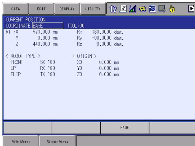
7. Set the recorded Rx, Ry and Rz values to {REF. ANGLE} on the tool angle monitoring condition file window.
