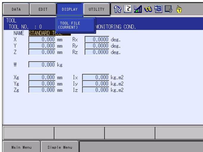
When verifying the current tool file against the tool file that was saved on the safety board, the comparison result of the following two tool files: the tool file that was last saved on the safety board and the tool file to use normally (TOOL.CND) is output to a concurrent I/O signal (specific output signal).
