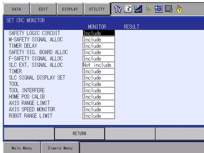
3. RESULT can be confirmed on the page of “Total safety number” on the TOTAL CRC CONFIRM window, on “SET CRC MONITOR” window, and by the specific output signal.
