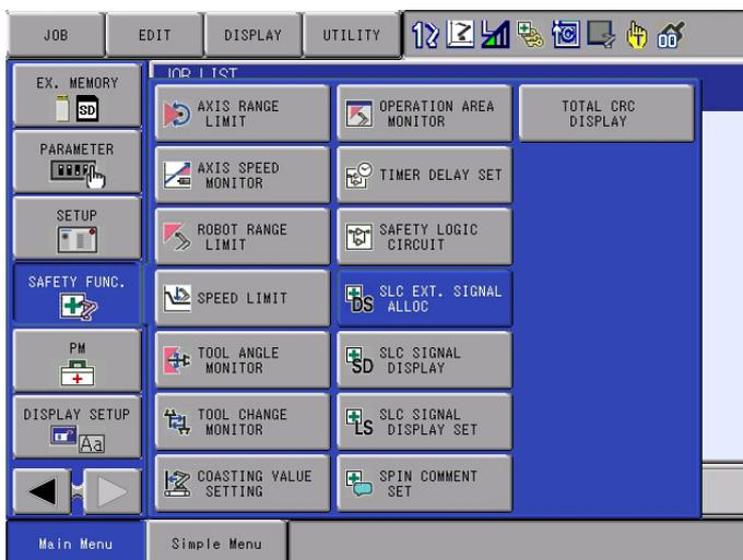
2. Select {SLC EXT. SIGNAL ALLOC} under the submenu.
