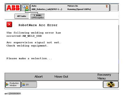
The user can tap **Move Out** to extract the tool from the partially welded part in increments. Tapping **Abort**, stops execution. Tapping **Recovery** menu will bring up the **Recovery** menu.
