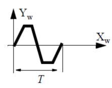
T = Weaving cycle time  $X_{w}$  f = Weaving frequency
