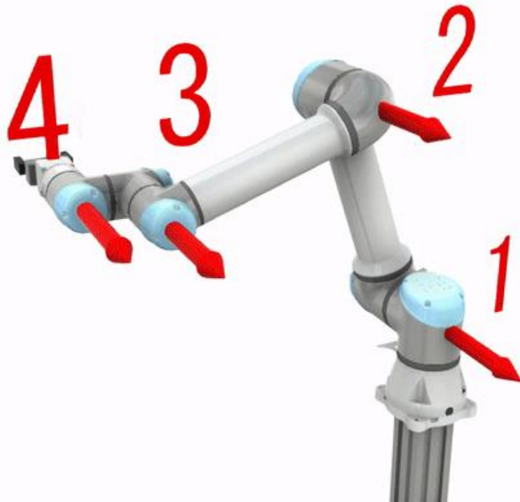
Figure 17 Wrist alignment singularity
