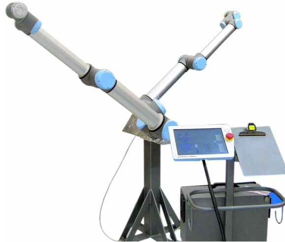
Figure 2.3: Mount the robots on the Calibration Horse, connecting the robot bases
