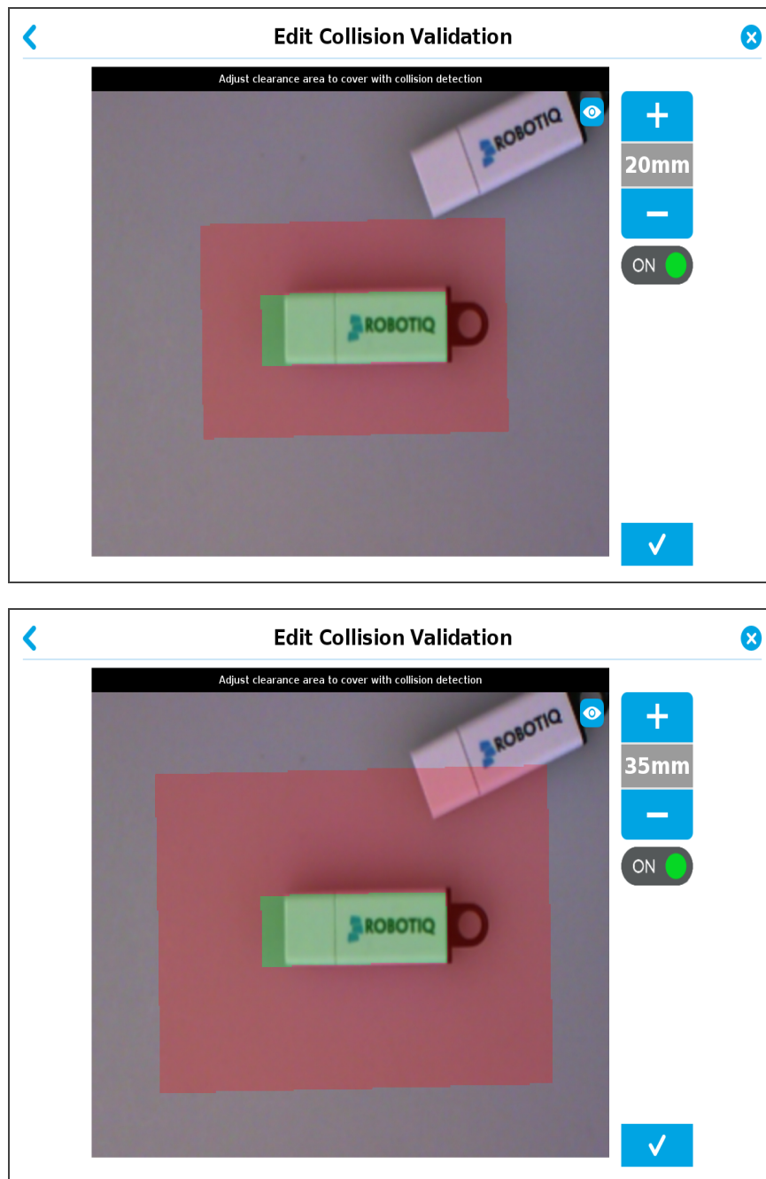
Fig. 4-57: Setting up the clearance perimeter.
