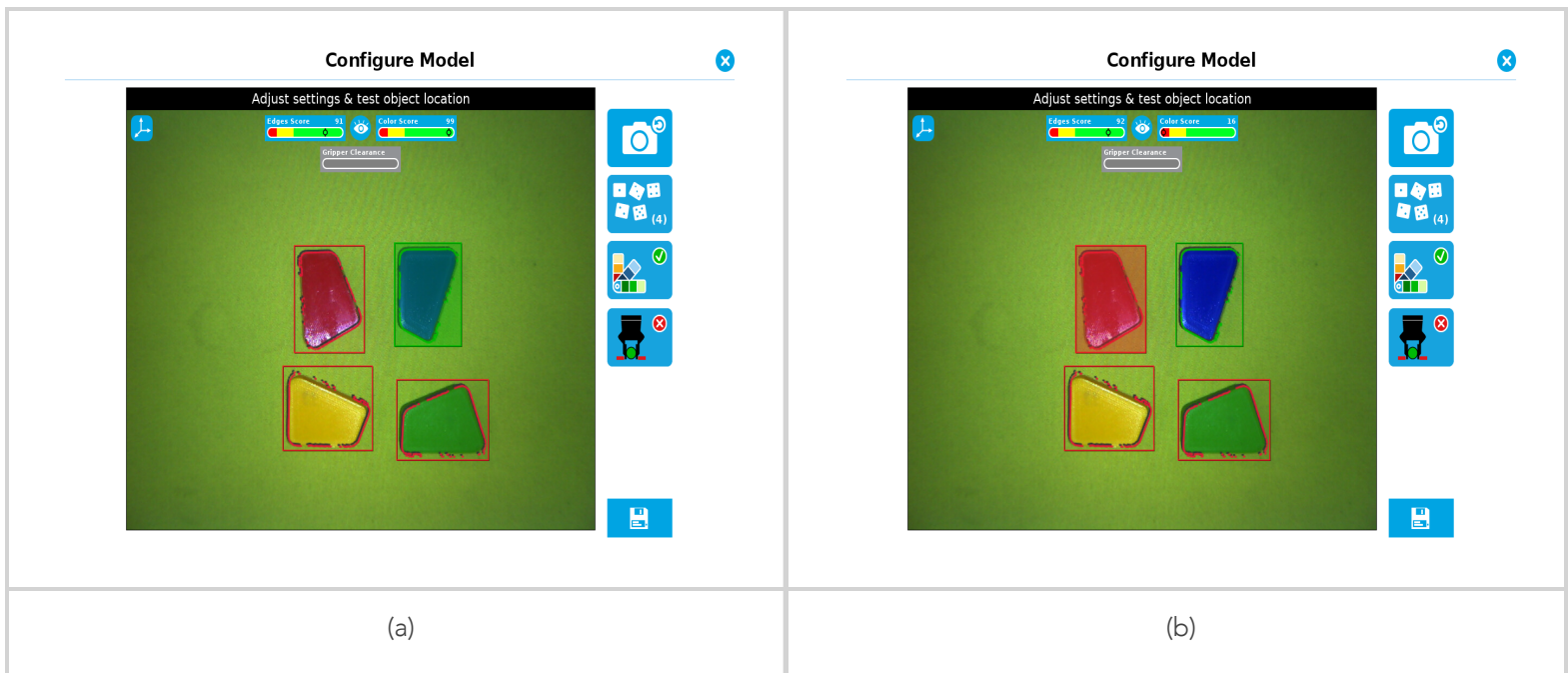
Fig. 4-44: Examples of Edges Score for (a) a blue part (b) a red part.
